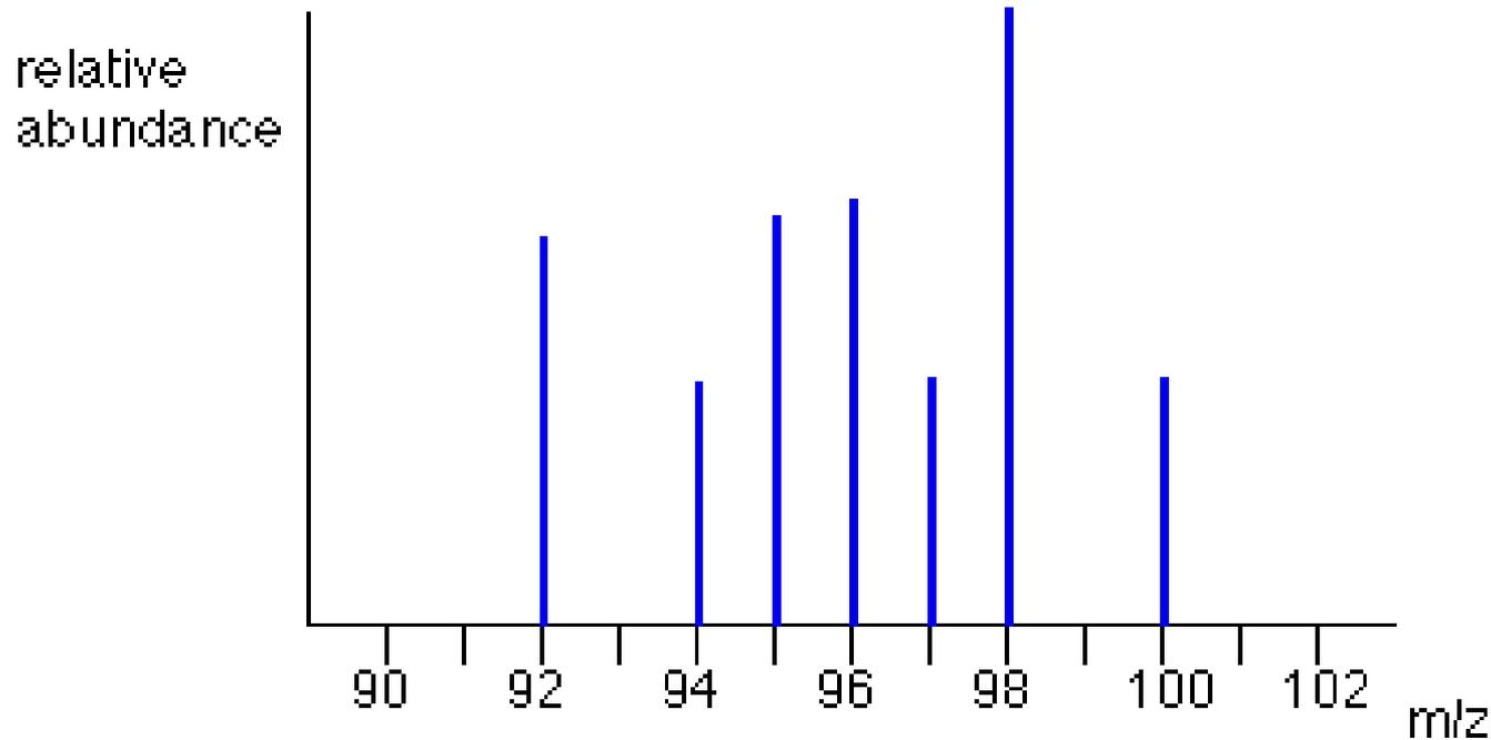
The vertical scale is related to the current produced at the detector. As you can see from the diagram, the commonest ion has a mass/charge ratio of 98.
