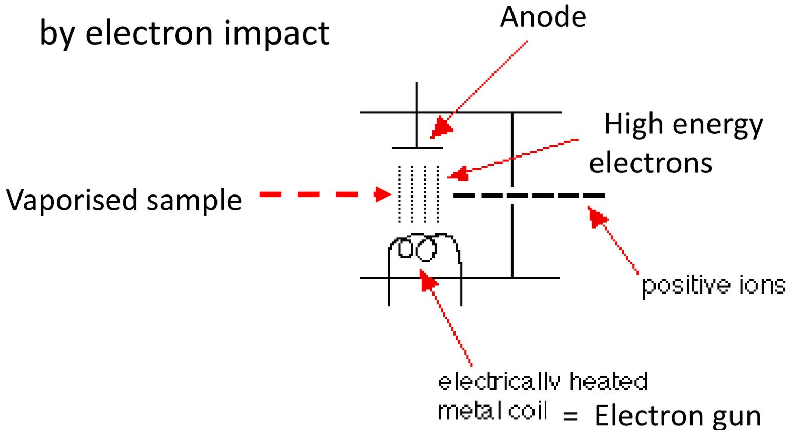
The atoms of the element are bombarded (hit) with a **stream of high energy electrons** fired from an electron gun.
